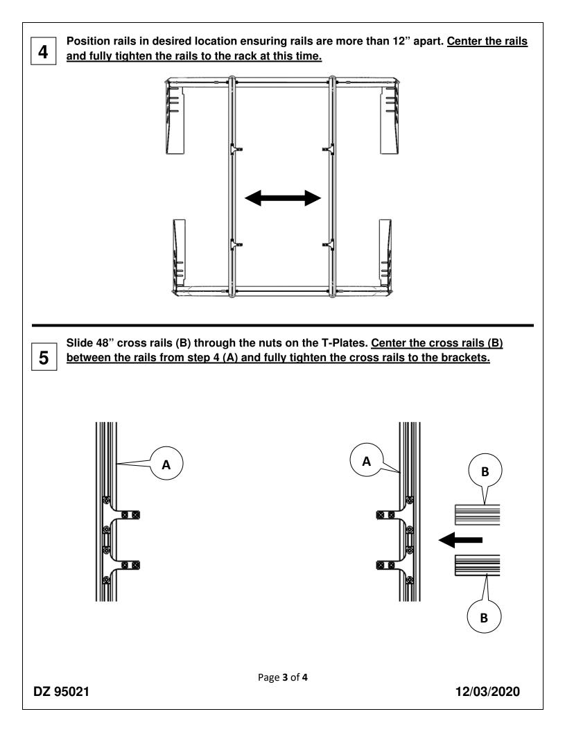
Slide cross rails (B) front to back to desired position ensuring rails are more than 12" apart. <u>Fully tighten brackets to Rail (A).</u>
